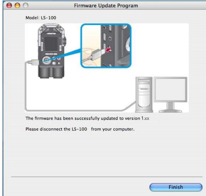
After "The firmware has been successfully updated to version 1.XX" is displayed, the recorder will reconnect itself to the computer. When the "Remote (Storage)" display appears on the recorder's LCD, proceed to step 11.
