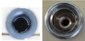
Fuse carrier without charring
