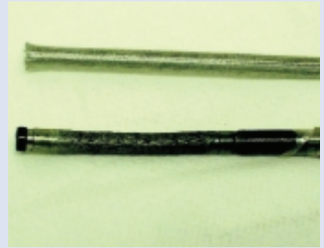
Fig. 9: Olympus braided mesh and bending section replacement repair
