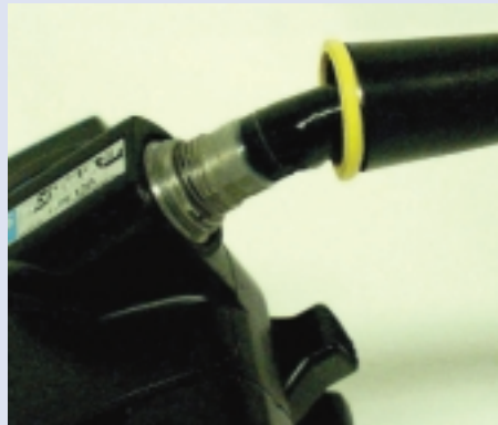
Fig. 4: Olympus light guide tube replacement repair
