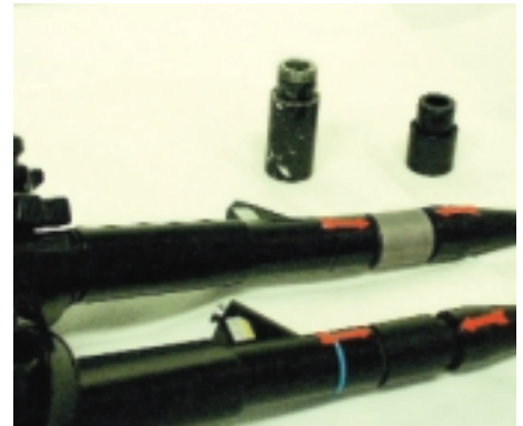
Fig. 5: Third-party repair using boot extenders
