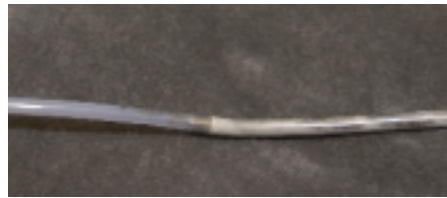
Fig. 1: Third-party spliced channel repair
