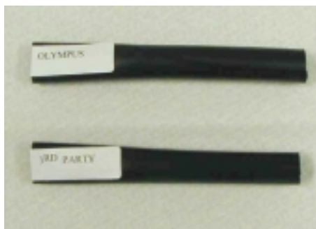
Fig. 11: Olympus-certified bending section covering compared to third party
