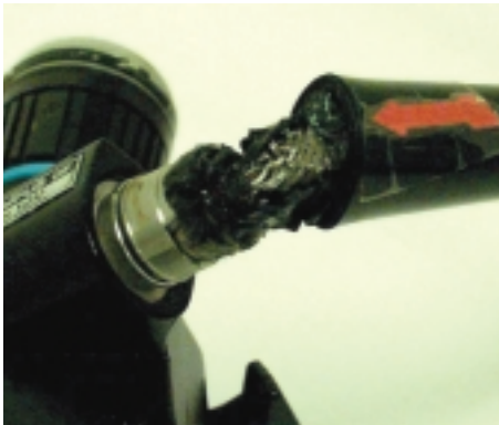
Fig. 3: Third-party light guide tube repair patch
