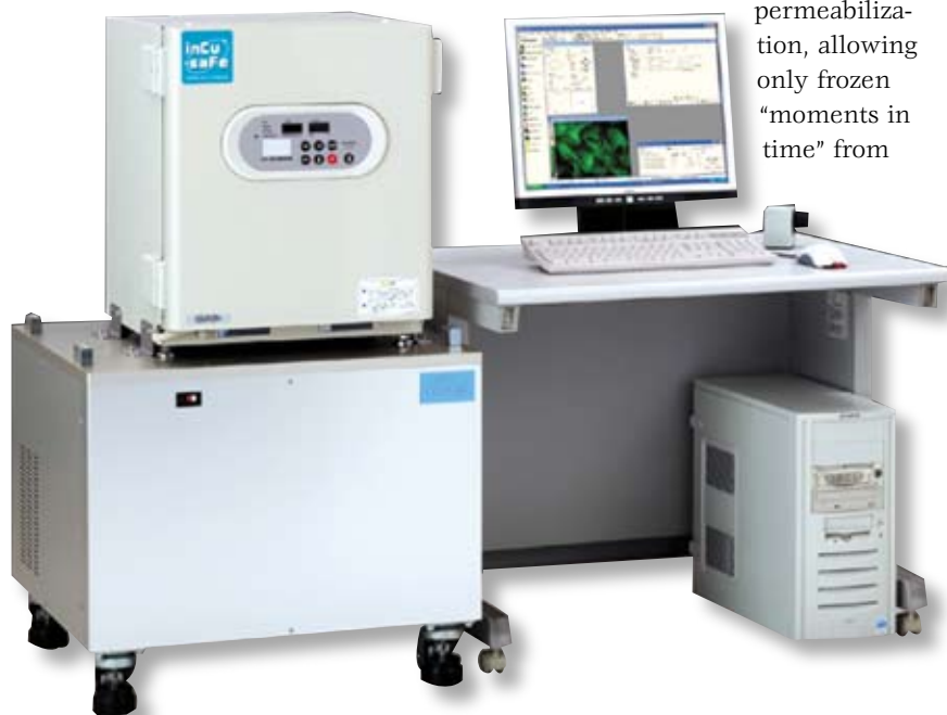
Left, Figure 1. Olympus VivaView FL Incubator Fluorescence Microscope, an ultra-long-term live cell incubation and imaging system that can handle observation of multiple locations in up to eight dishes simultaneously and handle high-resolution photomicrography. (Source: Olympus America Inc.)
